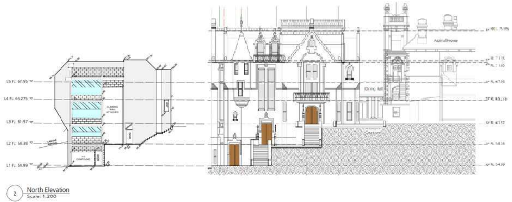
Figure 30. Existing vs Proposed Elevation – indicating no deep excavation. (JCA Architects, Drawing No. SSD1.02/17-201, Scale 1:200 @ A3)
